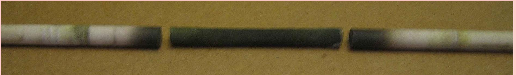
Fuel container after removal from the reactor tube. On each side, the ceramic filler inserts.
